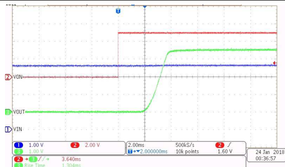
Figure 14. Turn On at 5 V (CT = 1000 pF)
