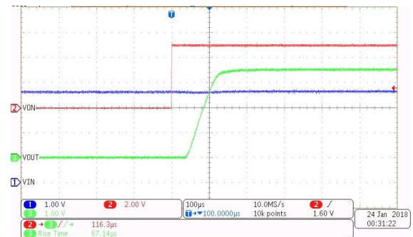
Figure 8. Turn On at 5 V (CT = Open)
